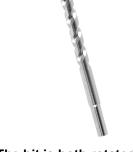
Masonry Drill Bits: Masonry bits typically are used with a hammer drill. The bit is both rotated and hammered into the work piece; the hammering breaks up the masonry at the drill bit tip, and the rotating flutes of the drill bit body carry away the dust. Rotating the bit brings the cutting edges onto a fresh portion of the hole bottom with every hammer blow. Hammer drill bits often use special shank shapes such as the common SDS type.
