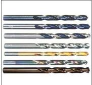
Twist Drill Bits: The twist drill bit is the type produced in largest quantity today. It comprises a cutting point at the tip of a cylindrical shaft with helical flutes; the flutes act as an Archimedean screw and lift swarf out of the hole.
