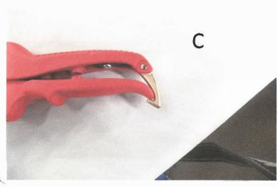
The handle lock in picture C holds the handle closed for storage.
