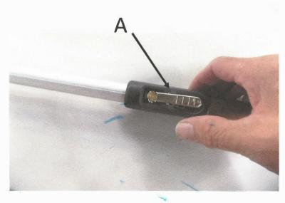
To extend pole, press the lever indicated by arrow in picture A down and slide pole up to the desired length. Make sure the pin in lever A locks into a hole. If not locked into the pole the handle will not open and close the blade.
