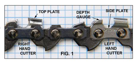
The cutting element has a profile that resembles the number "7"; its two surfaces, the top plate and the side plate, contain three different angles. The *top-plate angle* (Fig. 2: A) is the familiar 25-35 degree angle you see when you look down on the chain; the *top-plate cutting angle* (B) is the bevel on the underside of the top plate; the *side-plate angle* (C) is the beveled arc in the side plate.
