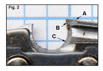
Getting the angles exactly right is not as important as removing all damage from the side and top plate and making sure the critical top corner is really sharp.
