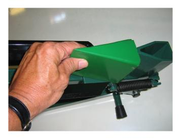
If the advancing ram interferes, slide it back just enough to facilitate installing the wedge. You are now ready to split your first log. The pressure from the log will fully seat the new wedge.
